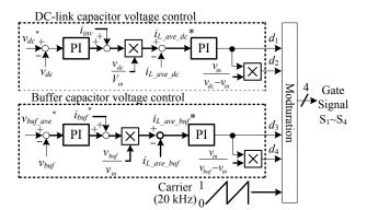
Fig. 3. Control block for DC link voltage and buffer voltage. Table 1. Circuit parameters of the prototype.
