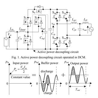
Fig. 2. Single-phase power pulsation compensation.
